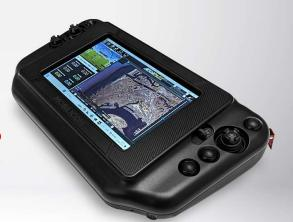
The Mobilicom 8" Controller Pro is a state-of-the-art Ground Control Station (GCS) designed to meet the rigorous demands of drone and robotics operations. This ruggedized, IP65-rated Tactical Mobile GCS delivers reliable performance in harsh environments, making it essential for military, industrial, and commercial applications. Its high-brightness display offers more screen real estate than smaller models, enhancing situational awareness while maintaining portability. The
